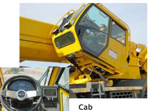
The Full Vision cab on the RT890E tilts up to 20° providing the operator additional comfort when working at long boom and extension lengths.
