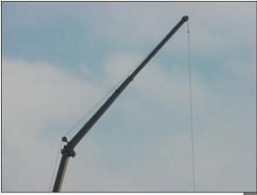
26 ft. - 45 ft. telescoping swingaway extension with offset up to 30° maximizes up and over capacity.
