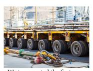
We transported the first new cold train module to the crude unit using its Goldhofer modular trailers.
