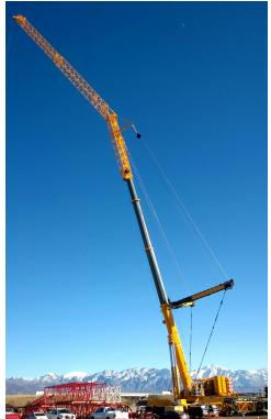
Mountain Crane is excited to introduce the newest member of the team! One of only four cranes like this in the US, this LTM 1750 9.1 crane has a lift capacity of 900 ton. assembly technology and easy of mobility, making it ideal for tight, small compact spaces, and windfarms. With less build space, quicker assembly time, and fewer load trucks, this crane is ideal for your next heavy lift.
