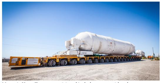
Mountain Heavy Transport participated in the largest ever pick and transport at Energy Solutions in Clive, UT. The piece was a 1.2 million pound steam generator that was offloaded from rail, transported to a containment cell, and set on to sand saddles. We utilized a 700 ton gantry and 20 lines of Goldhofer SPMT for the project. The job involved months of planning and ultimately a lot of hard work.
