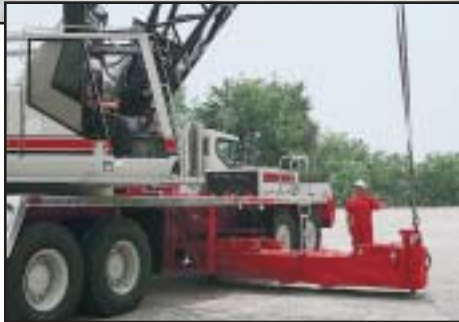
The front outrigger box can be easily removed for transport in locations with severe weight restrictions.
