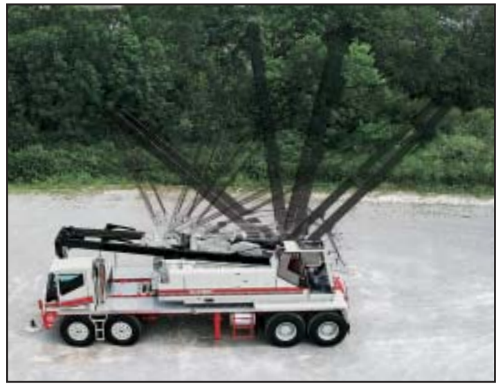
HC-238H II base machine travels at under 85,000 lbs (38 555 kg) and the HC-248H travels at under 93,000 lbs (42 185 kg).
