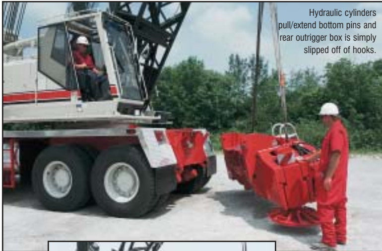
The front outrigger box can be easily removed for transport in locations with severe weight restrictions.
