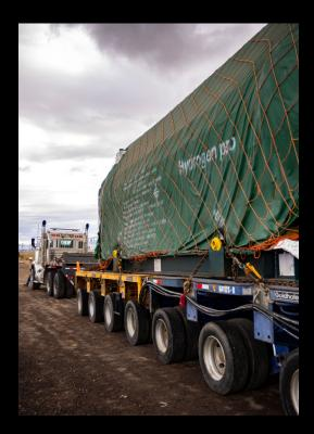
When the crane can only get your load so far, it's time to hand it off to Mountain's Special Projects Team. We have specialty rigging and transport equipment that can complete any job from start to finish. Recently, our team lifted 40 electrolyzers (weighing 165K lbs each) off the rail line and onto 6 lines of THP Goldhofer trailer. Once the Goldhofer moved the units across the laydown yard, the crane picked each unit and set
